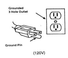
This machine is for use on a nominal 120 – volt circuit and has a grounding plug that resembles the plug illustrated in the figure below. Make sure that the machine is connected to an outlet having the same configuration as the plug. No adapter should be used with this machine.
