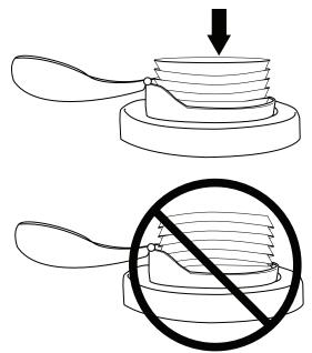
While holding lids in place, close lid dispenser door, snapping latch securely in place.
