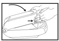
4. Close cover. **NOTE:** Pressure plate carriage will automatically release when cover is closed, applying pressure to napkins.
