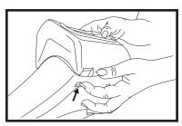
2. Locate 2 tabs under front of face and depress upward into base one at a time.
