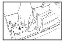
Using thumb hold, move pressure plate to back of unit until locking tabs engage.
