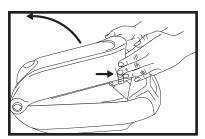
Open cover by pressing in on both sides of cover and swing cover up and back.
