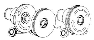
Always attach brush by hand. **Never** by placing machine over an unattached brush and starting machine to lock brush. This will **cause gear box damage not covered by warranty**.
