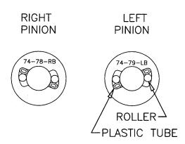
**NOTE!** The right and left side are determined from the operators position.
