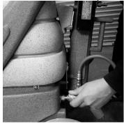
4. Connect the power cord on the heater (#4 on page 7) to the female twist-lock plug on the machine (#8 on page 6.)
