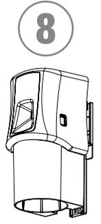
Replace cover on dispenser. Line up two slots on the back of the dispenser with the two ribs on the backplate. Slide down until you hear a 'snap' to ensure the dispenser is securely locked into place.
