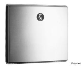
Rough Wall Opening 11-1/4" (285mm) wide 9-1/2" (240mm) high 4" (102mm) minimum recessed depth
